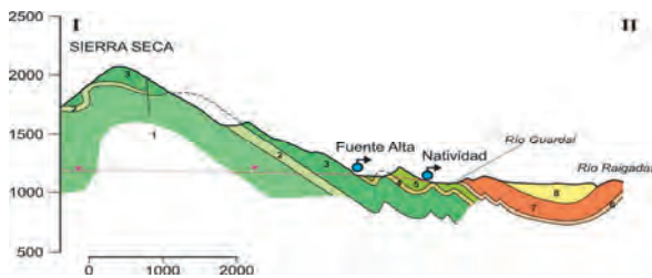
Figure 2: Hydrogeological cross-section. Located in Fig. 1.
