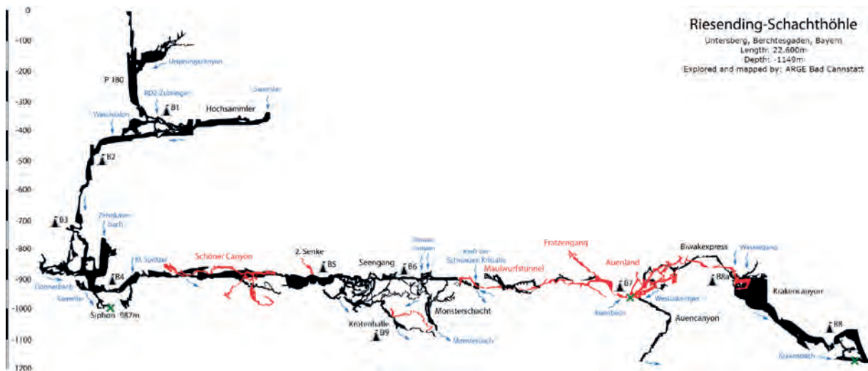
Figure 2: Vertical section of Riesending, with major waterways (blue) and the location of water pressure gauges (green).
