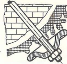
Fig. 8 Yielding securing of detached dripstone by rock anchor
