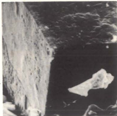
Fig.2- The Faggeto Tondo cave. A: gypsum crystal inside a corrosion hole of the limestone wall (x160); B: fluorite crystals replacing the limestone (x350); C: corroded fluorite crystal (x1800) (Photo P.Ferrieri)
