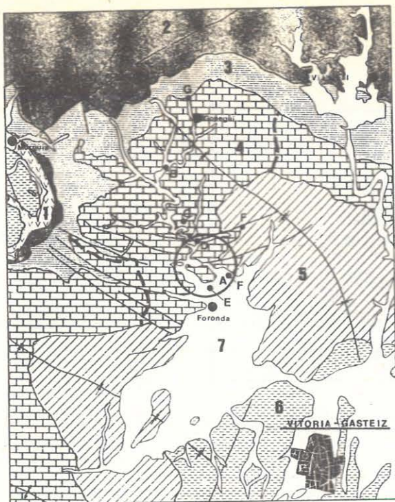
Fig. 2 Geologic and hydrogeologic context. 1. Clay & Gypsum; 2. Sand-stone; 3. Lower marl; 4. Limestone (Karstic aquifer); 5 - 6. Upper marl; 7. Detritic materials of the river; A. Main discharge area; B. Bocarrón de Zaragoza Cave - Main drain in the Zubialde bed-river; C. Zambolino Cave; E. Ugau spring; F. Industrial well (2,000 m 3 /day); G. Drains in contact with limestones; H. Echávarri-Viña I well.
