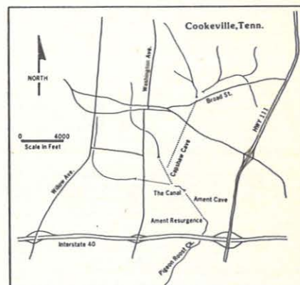
Figure 2. Locations and hydrologic relationship of the Capshaw and Ament Cave systems, in Cookeville, Tennessee, USA. Dotted lines indicate straight-line subterranean flow paths.
