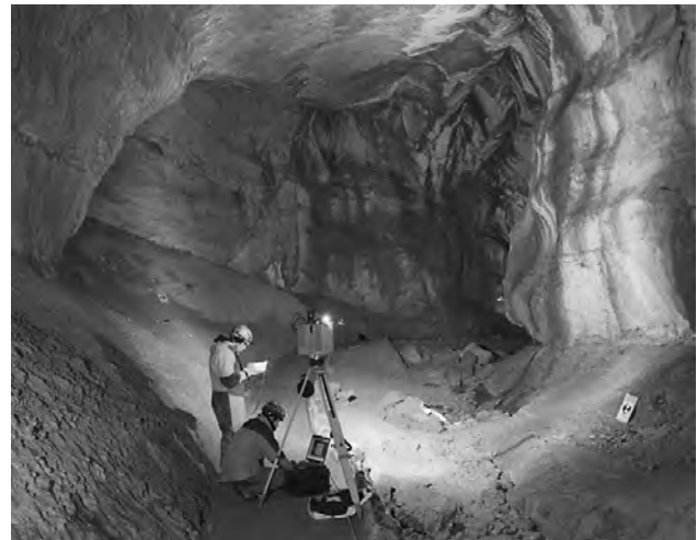
Figure 1. Performing the terrestrial laser scan in Paläotraun.
