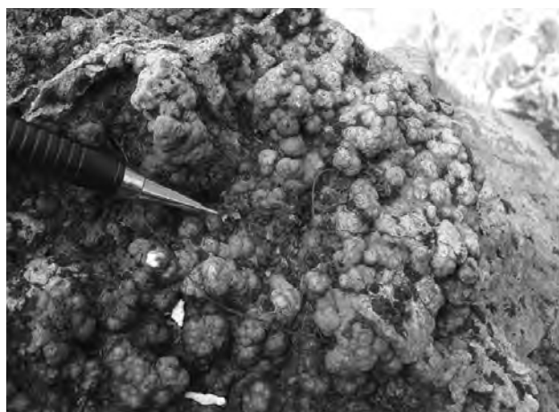
Figure 5. Botryoidal collophanite on the top of main ore body of Itataia deposit.
