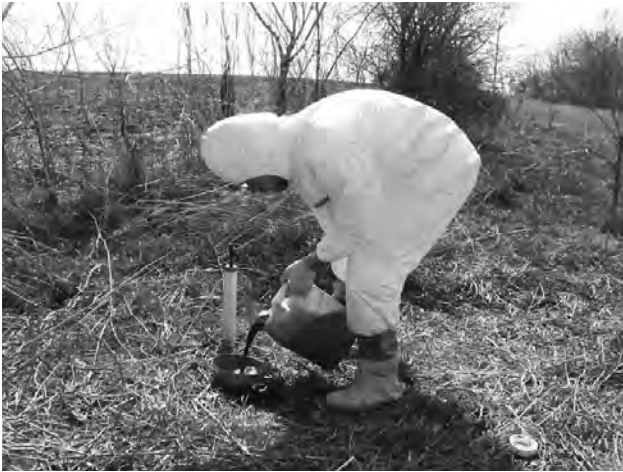
Figure 8. Injecting fluorescein dye into drilled hole in the soil column.
