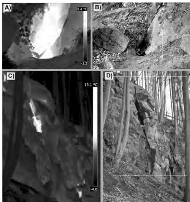
Figure 2. Results of the IRT survey at the Křížový Site: A) IRT image of the entrance of the Zbojnická Cave, B) BW photography of the same area, C) IRT image of a toppled rock column indicating open cracks behind it, D) BW photography of the same area.
