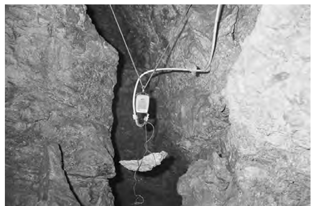
Figure 3. Anemometer/Datalogger in Loferer Schacht.
