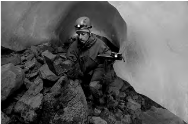
Figure 3. Using an Xbox Kinect to survey a cave. Photo: Jason Gulley.
