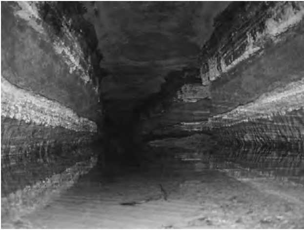
Figure 6. A passage flooded by water in a lignite mine.
