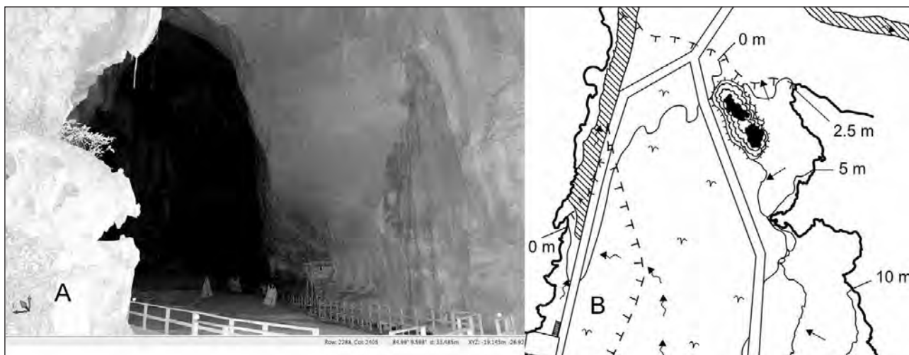
Figure 2. (a) 3D point cloud in FaroScan, Simud Hitam entrance. (b) Plan of Simud Hitam based on LiDAR data, with centimeter-precision wall detail.
