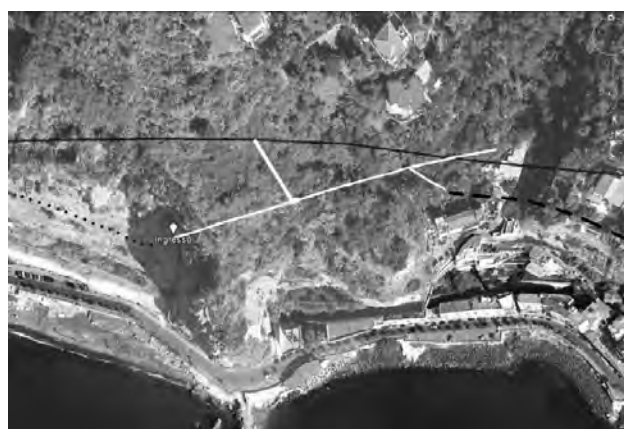
Figure 4. La Pietra. White: the cave; dashed black: inferred upstream aqueduct; dotted black: the destroyed downstream aqueduct; solid black: railway tunnel.
