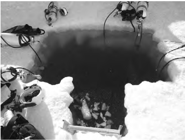
Figure 9. The temperatures, both topside and in the water, are so extreme that diving regulators need to be submerged at all times to prevent them from freezing.
