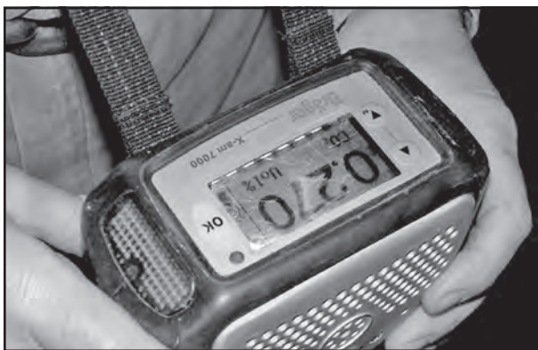
Figure 4: X-am 7000 by Draeger, infrared portable device.
