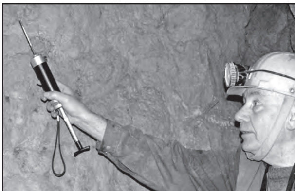
Figure 3: Gastec pump detector giving a direct reading of CO 2 concentration (Ek & Gewalt, 1985).
