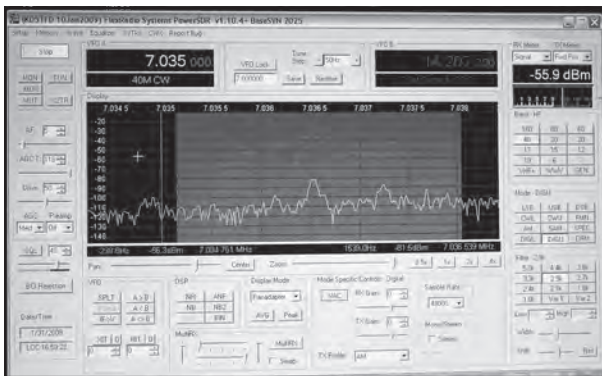
Figure 6: Display for Software Defined Radio using PowerSDR.
