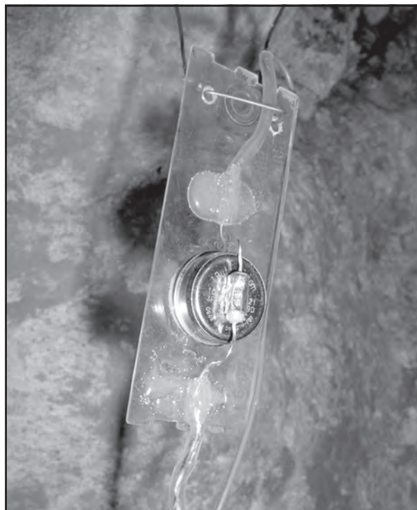
Figure 1: Low-cost airflow data logger based on the hot-wire anemometer principle that uses a resistor thermally coupled to an iButton.
