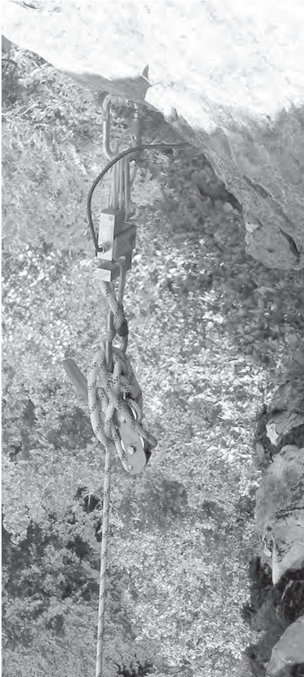
Figure 2: The top anchor and the dynamometer.
