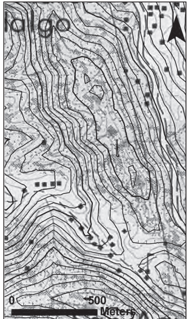
Figure 4: SRTM data-derived elevation contours laid over the Huautla 1:50,000 quadrangle topographic map (Mexico).
