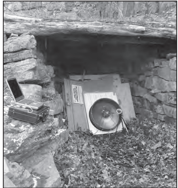
Figure 1: The rectangular doorway Butler Cave's Sofa Entrance has been sealed around a fan. The fan blows alternately in and out of the cave in even intervals. A signal is sent from the fan to a recording data logger when the fan changes direction.
