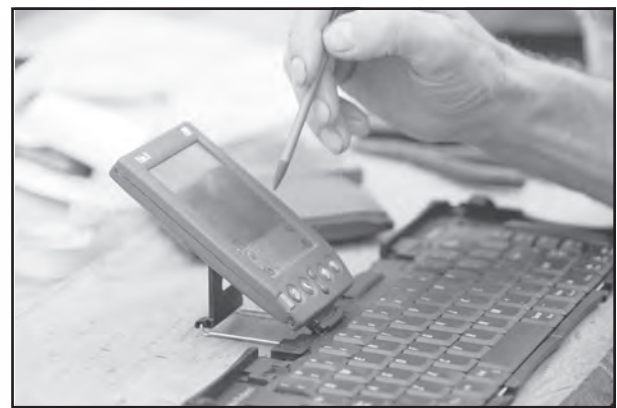
Figure 3: A Palm PDA mounted on a foldable keyboard. Unknown photographer.
