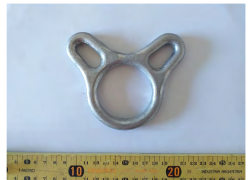
Fig. 4: Osito F (cast, deburred and polished finish). PHOTO D. MENDY
