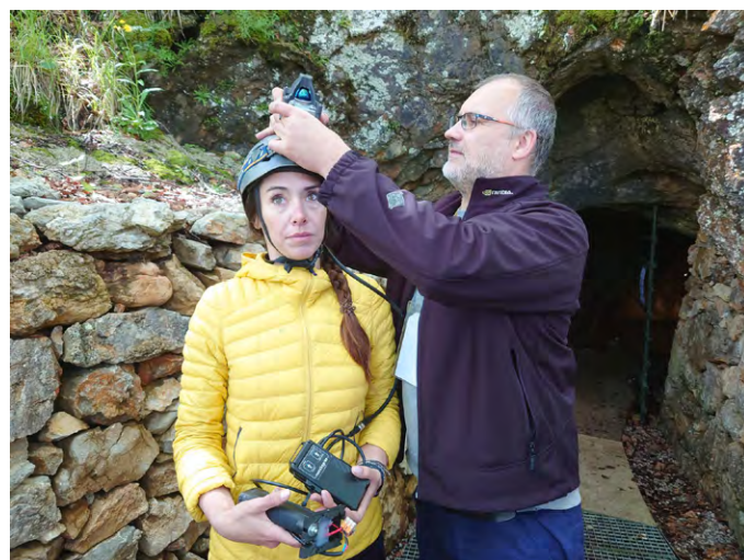
Demonstration of setting up a 3D LiDAR scanning custom-made device. PHOTO: BORIS STANOJEVIĆ
