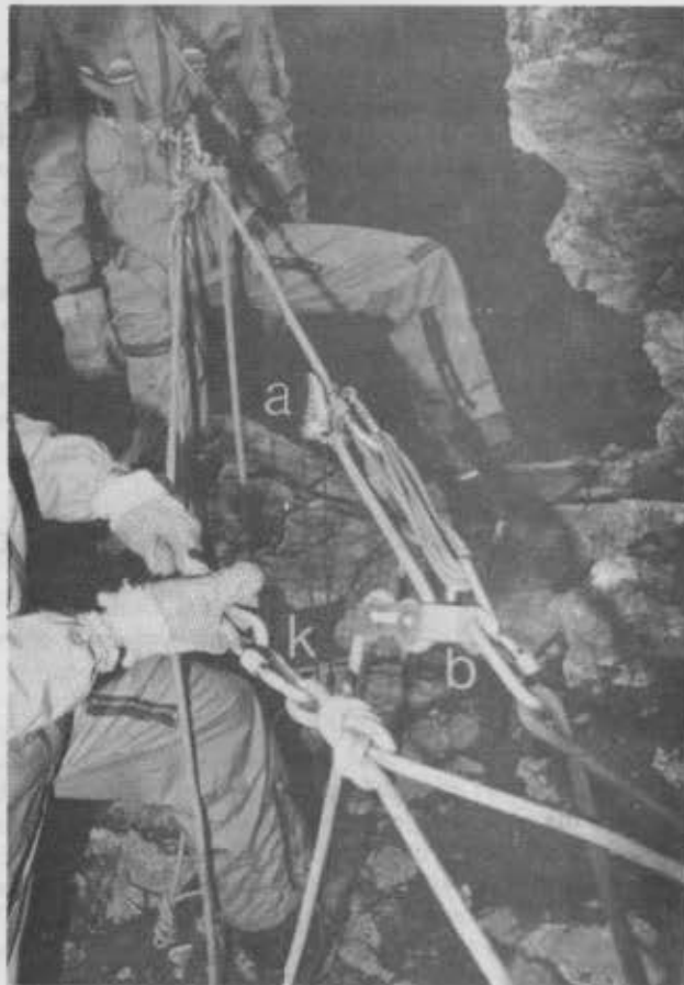
3. a = shunt Petzel; b= descendeur Petzel k = karabiner
