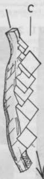
Figure 1B. If rhombohedrons are stacked in other growth directions (arrow) than parallel to the crystallographic C-axis, pseudo-tetragonal cross-sections appear. Often the rhombohedron faces are developed on one side of the crystal only.
