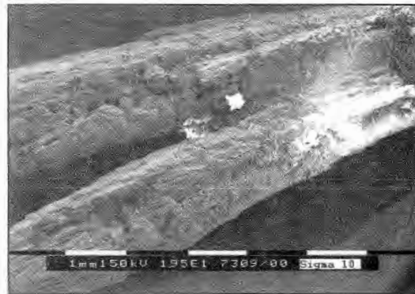
Figure 6: "Twig" (SEM photo). Aragonite laths coated with Mg-rich minerals.
